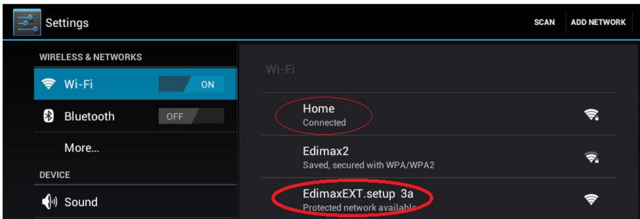
If the extender is in default settings, you will see the wireless network "EdimaxEXT.setup". Tap on "EdimaxEXT.setup" to connect to it. If you already setup the extender to join your existing wireless network, you will see the \_2EX wireless network. Select the extender's wireless network to connect to.
