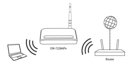
Position the device in a location for optimal wireless extension, such as the middle of your house. You can connect to the device wirelessly by searching and connecting to the device name you set up.
