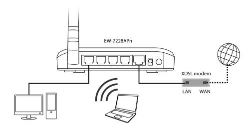
Connect one port of the device to your router or xDSL modem. You can now connect to the device through a wired connection by connecting your computer to it with an Ethernet cable, or connect to the device wirelessly by searching and connecting to the device name you set up.
