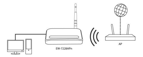
Connect one port of the device to the appliance you wish to connect to the Internet wirelessly, such as a computer, game console, or smart TV.
