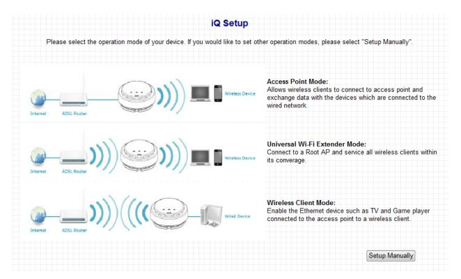
The default mode for the device is Access Point Mode. For Universal Wi-Fi Extender Mode and Wireless Client Mode, please refer to the user manual in the enclosed CD.
