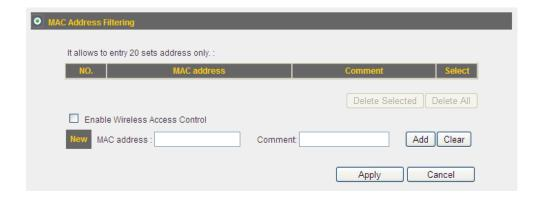
To enable MAC address filtering, please check 'Enable Wireless Access Control' box in this page, the descriptions of other setting items are listed as follow:
