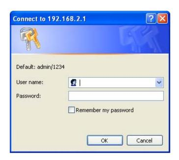
NOTE: If you cannot access the broadband router's web-based configuration interface, the IP address you have inputted may be incorrect. If you have previously changed the router's IP address, please input the one you have designated.
