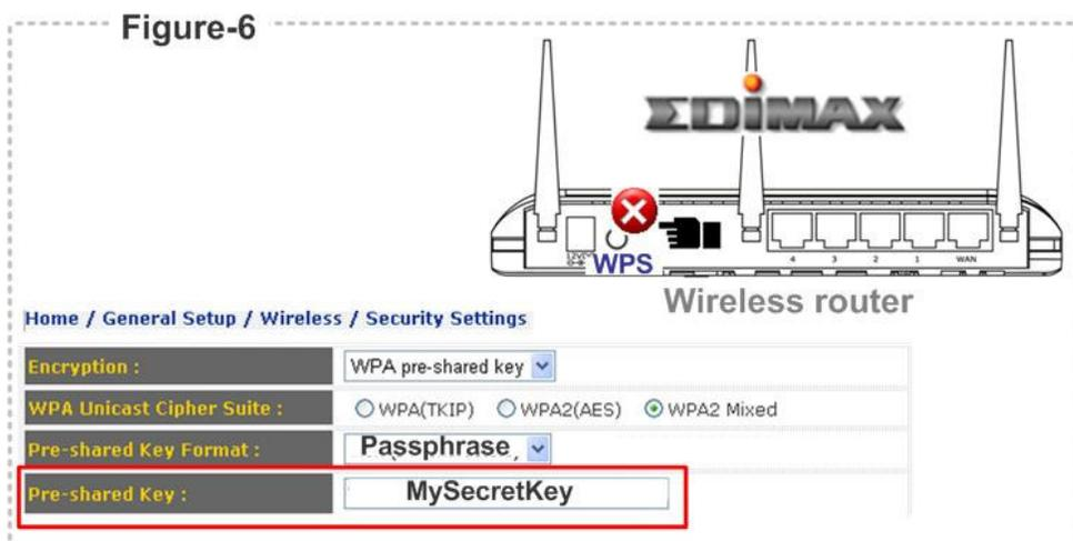
The same key is also used for wireless cards having WPS button to form a wireless security connection. But the difference is that wireless router will not ask such key.
