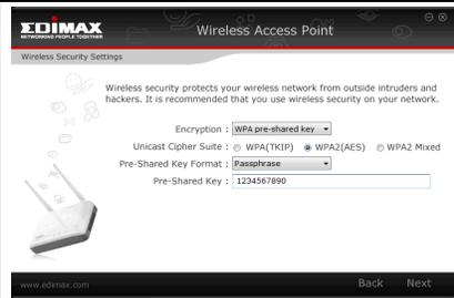
Enter your correct wireless security passphrase key. The security password must be the same with the wireless password of your original Wi-Fi network. Please note the password is case sensitive.
