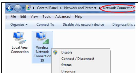
If you see **Wireless Network Connection** icon in **Network Connection** window, **right** click on **Wireless Network Connection** and click on **Disable**. The wireless network connection will be disabled.
