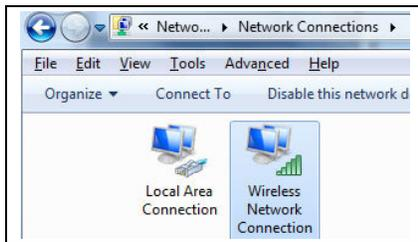
Double click on the **Wireless Network Connection** icon to get into Wireless Network Connection Status window.
