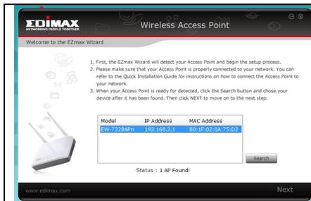
The Setup Wizard finds the Wireless Access Point and shows its current IP address 192.168.2.1. Click on Next.
