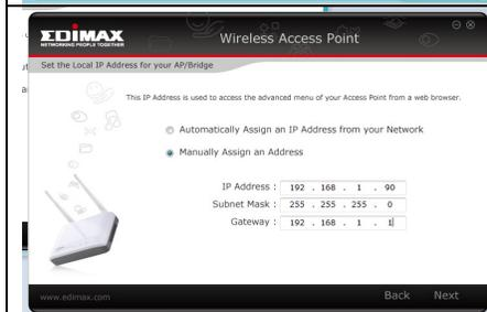
Based on information gathered in Step 1, the existing wireless network uses 192.168.1.x network. I know no device will use 192.168.1.90 so it will be the new IP address to Access Point.
