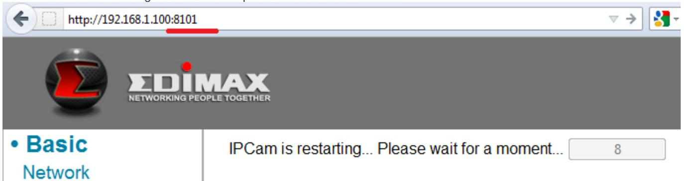
Login to the router's setup page. Setup the port forwarding for port 8101 to IC-3015Wn.
