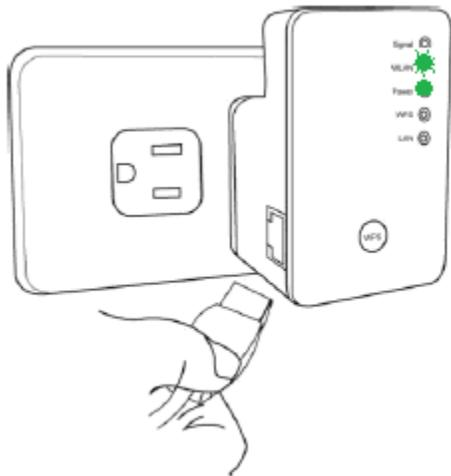
3. Connect the Ethernet cable to LAN port of your computer.
