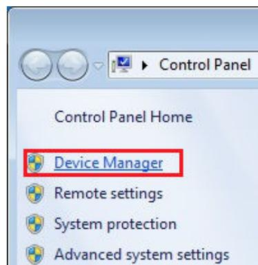
2. Inside Device Manager, expand the list of **Network Adapters** . If you see the wireless adapter is listed in **Network Adapters**, its driver could have been installed properly. However, if you see **802.11n WLAN Adapter** is listed under **Other Devices**, you will continue to install the driver manually.
