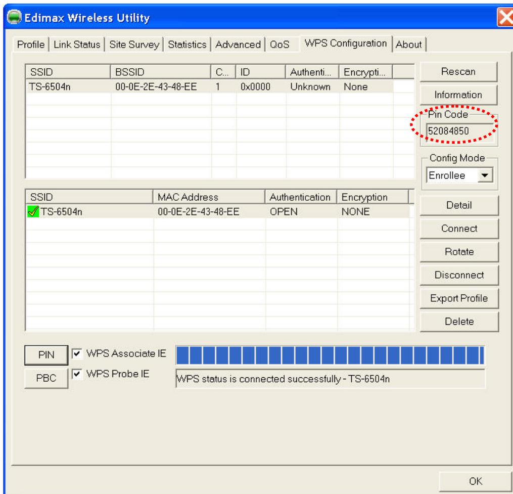
The PIN number of your wireless network card is an eight-digit number located at the upper-right position of configuration utility. Remember it, and input the number to your wireless access point as the WPS PIN code (Please refer to the user manual of your wireless access point for instructions about how to do this).
