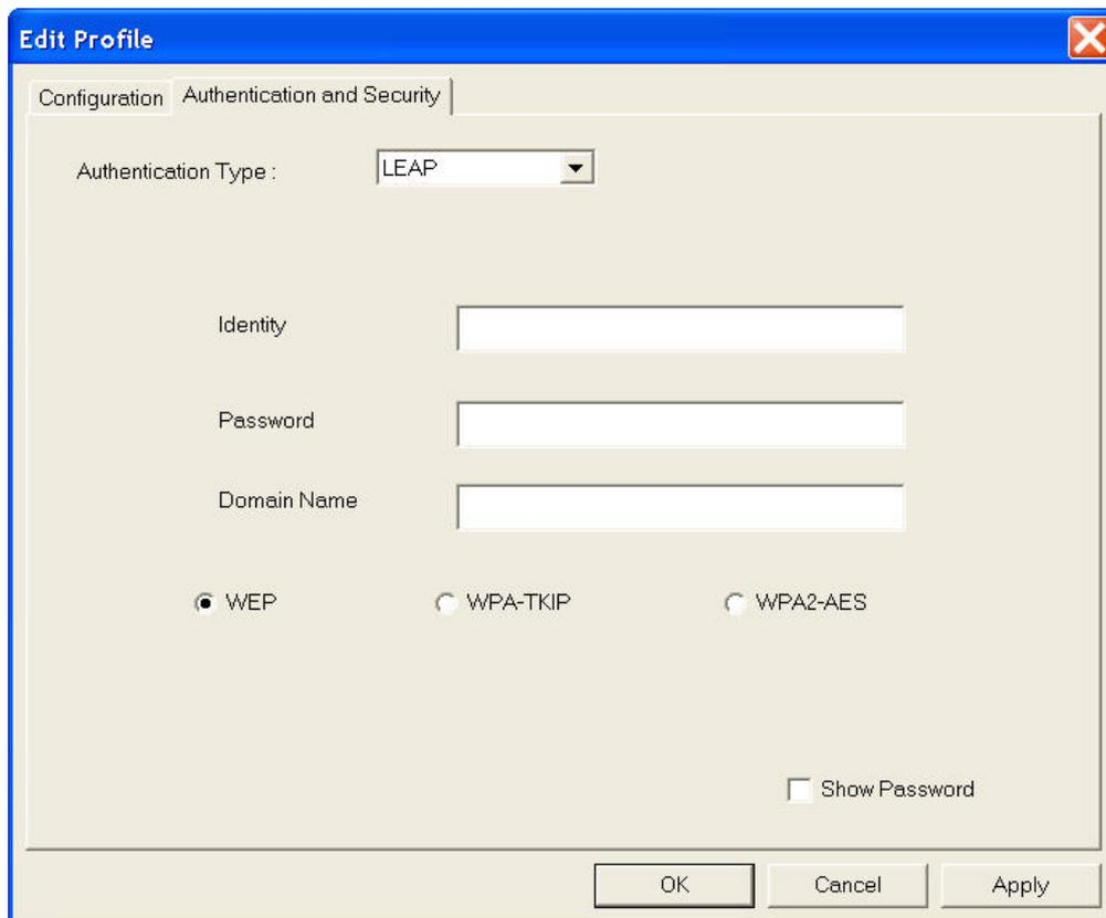
**Encryption:** *Select the encryption type of the wireless access point or wireless device you wish to connect. If you're adding a profile from an existing access point or wireless device, the value will be selected automatically, and please do not modify it.*
