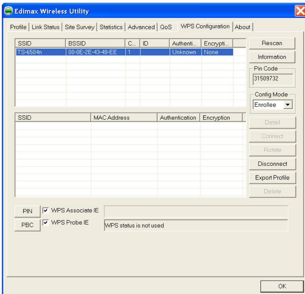
3. Set 'Config Mode' to 'Enrollee', and then push the 'WPS' button on your wireless access point (the button used to activate WPS standby mode may have another name), or use other way to start WPS standby mode as the instruction given by your wireless access point's user manual.
