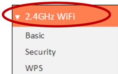
The “2.4GHz WiFi” & “5GHz WiFi” menu allows you to configure SSID and security settings for your Wi-Fi network along with a guest Wi-Fi network. WPS, access control and scheduling functions can also be managed from here. You can quickly enable/disable the 2.4GHz or 5GHz Wi-Fi from this screen.
