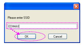
5. If the wireless access point uses encryption, you have to input WEP passphrase or WPA preshared key. Please ask the owner of the wireless access point you want to connect, and input the correct passphrase / preshared key here, then click 'OK'. If the value you inputted here is wrong, you will not be able to connect to this wireless access point.
