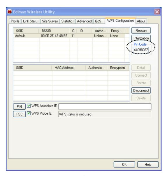
The PIN number of your wireless network card is an eight-digit number located at the upper-right position of configuration utility. Remember it, and input the number to your wireless access point as the WPS PIN code (Please refer to the user manual of your wireless access point for instructions about how to do this).
