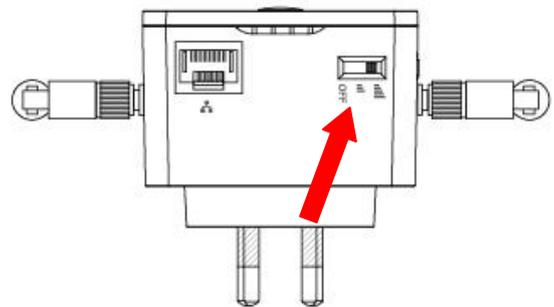
If you are using the extender in a small or medium sized space, you may not need the full power of the wireless radio. Try it, and determine if you still have sufficient Wi-Fi coverage using green mode. If so, you can save some energy.
