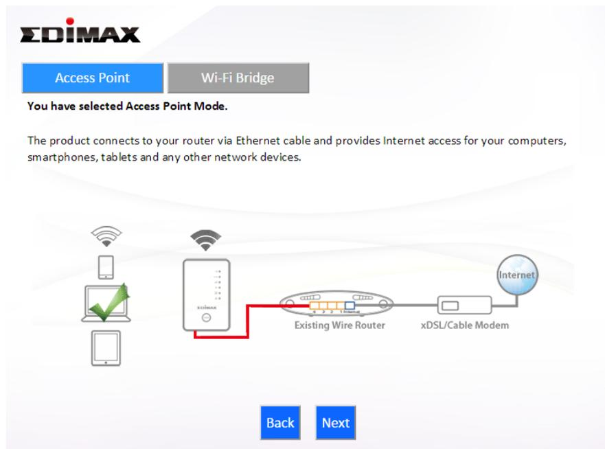
2. Connect the network port of your EW-7478AC to the LAN port of your existing router using an Ethernet cable, then click “Next”.
