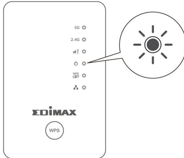
**3.** Use a Wi-Fi device to connect to the SSID “EdimaxEXT.Setup \*\*”. The last two \*\* characters are unique according to your device.
