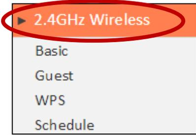
The “2.4GHz Wireless” & “5GHz Wireless” menu allows you to configure SSID and security settings for your Wi-Fi network along with a guest Wi-Fi network. WPS, access control (in access point mode) and scheduling functions can also be managed from here.
