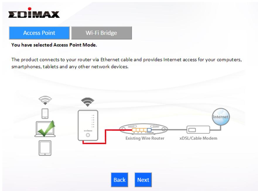
2. Connect the network port of your EW-7438AC to the LAN port of your existing router using an Ethernet cable, then click “Next”.
