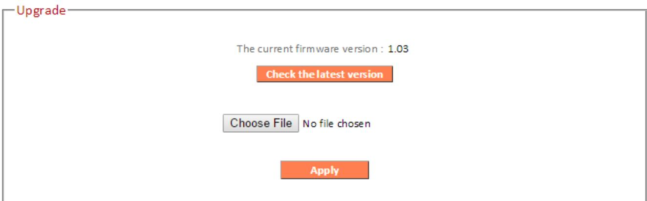
Click the orange **Check the latest version** button to open a new screen and automatically upgrade firmware to the latest version. Click **Firmware auto-upgrade** to begin the process or click **Save as file** to save the new firmware file to your computer and upgrade manually later.
