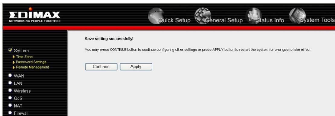
Press 'Continue' to save the settings made and back to web management interface; press 'Apply' to save the settings made and restart the router so the settings will take effect after it reboots.
