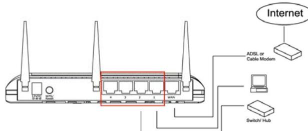
3. Connect the D/C power adapter to the wall socket, and then connect it to the 'Power' socket of the router.
