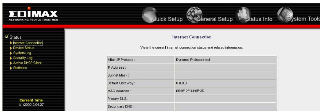
The screenshot shows the EDIMAX web management interface. The top navigation bar includes 'Quick Setup', 'General Setup', 'Status Info', and 'System Tools'. The left sidebar shows a 'Status' menu with options: Internet Connection, Device Status, System Log, Security Log, Active DHCP Client, and Statistics. The main content area is titled 'Internet Connection' and contains a table with the following data:
