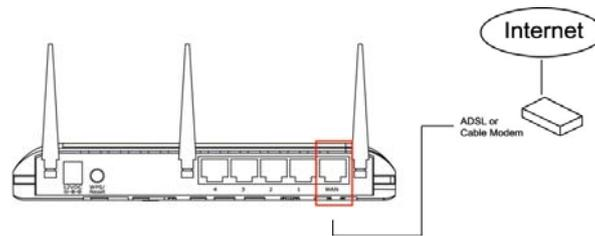
2. Connect all your computers, network devices (network-enabled consumer devices other than computers, like game console, or switch / hub) to the LAN port of the router.
