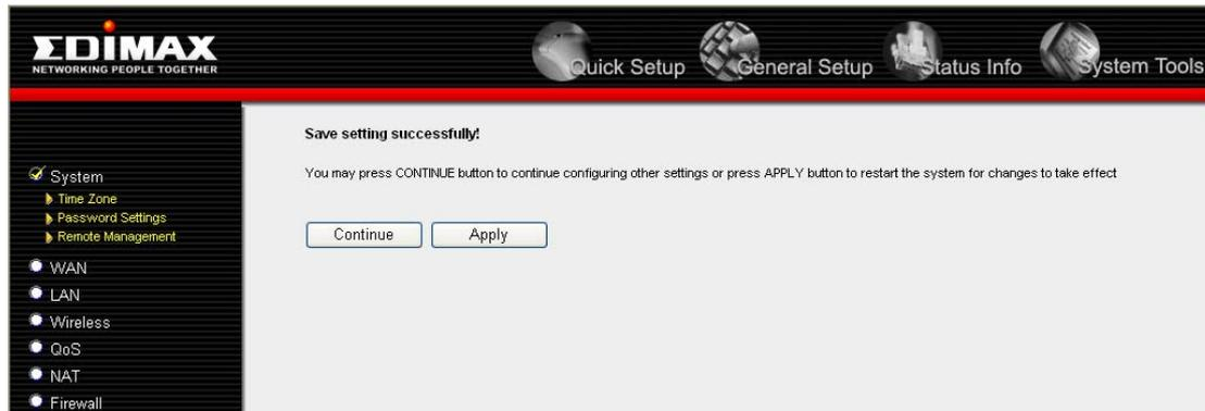
Press 'Continue' to save the settings made and back to web management interface; press 'Apply' to save the settings made and restart the router so the settings will take effect after it reboots.
