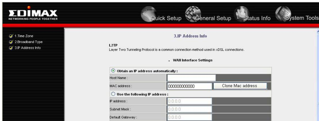
Please select the type of how you obtain IP address from your service provider here. You can choose ‘Obtain an IP address automatically’ (equal to DHCP, please refer to ‘Cable Modem’ section above), or ‘Use the following IP address’ (equal to static IP address, please refer to ‘PPPoE xDSL’ section above).
